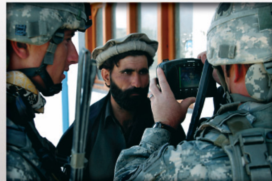
Lt. Marione watches his sergeant take a retinal scan in a process of registering village leaders. The portable camera also takes fingerprints and records biographical information.
